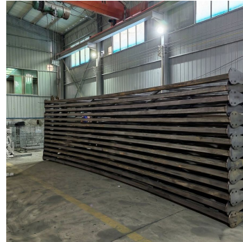
In-house welded steel trusses
