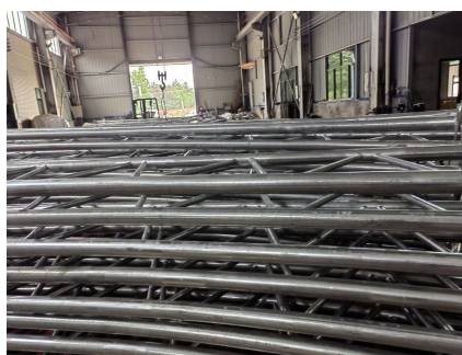
Galvanized tube trusses
