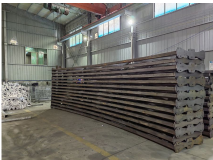
Welded truss sections
